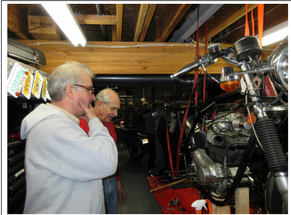
Tom Weisel and Bob Gilfillan study a 74 Commando hung from the ceiling like a slab of meat. The engine and transmission are in the frame but everything is floating. There is a problem with the replacement adjustable isolastic mount. Problem solved.
